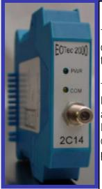
The 2C14 Module provides electrical interface for Modicon Remote I/O by conditioning the electrical signals supplied to and from Modicon equipment for transmission over the fiber optic network.
